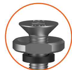
Collar with across flats for use with open end spanner.
