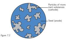
In the case of corrosion through galvanic cells, the most inert metal or particle is always a cathode, the most reactive one is always an anode.
